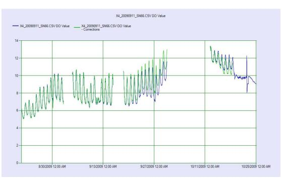
Figure 1. Dissolved oxygen record from Eureka Midges installed in the Moose River at CSAH 54 north of Grygla.
